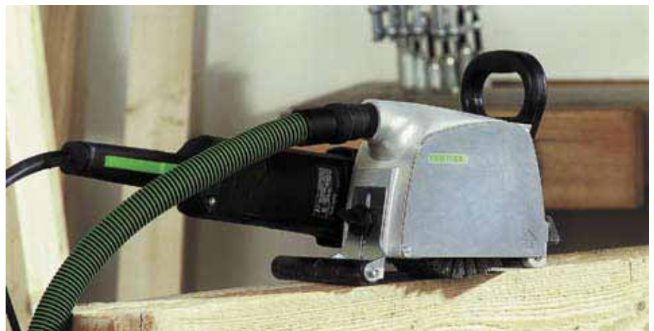
You can texture wooden surfaces quickly and easily with the RUSTOFIX brush machine – ideal for renovating old buildings and restoring timber.
